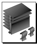
High power dissipation, extruded heatsinks designed to accommodate one or more TO220 or TO218/TO3P (TO247AD) packages via a clip retaining feature (clips available separately). Shaped to minimise board space, with a threaded slot provided to aid assembly. Choice of length.
