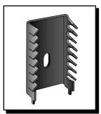
Tall twisted vane heatsinks with integral fixing tags and a slotted hole to accommodate a variety of plastic packages including TO220, TO218/TO3P (TO247AD) etc. (as illustrated) or TO202 (with cut-out).
