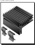
High power dissipation, extruded heatsinks designed to accommodate one or more TO220 or TO218/TO3P(TO247AD) packages via clips (available separately) or a threaded slot. Shaped to minimise board space by overhanging adjacent components. Additional threaded slot in base aids assembly. Choice of length.
