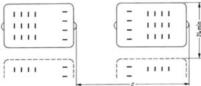
When mounting cradle relay P consideration should be given to magnetic fields. Strong DC magnetic fields, possibly caused by adjacent relays, and large iron masses are the most common causes of interference. Experience has shown that under normal operating conditions the minimum spacings specified for cradle relay P are sufficient to prevent cross interference.
