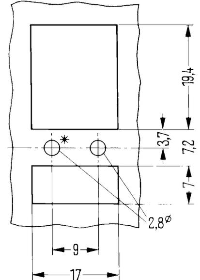
\*) This hole is omitted when the mounting hole layout is intended for the socket.
