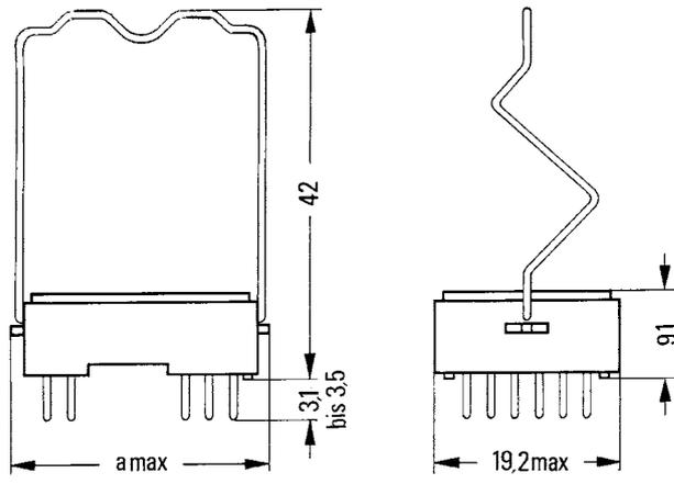
with hold-down spring for cradle relay W
