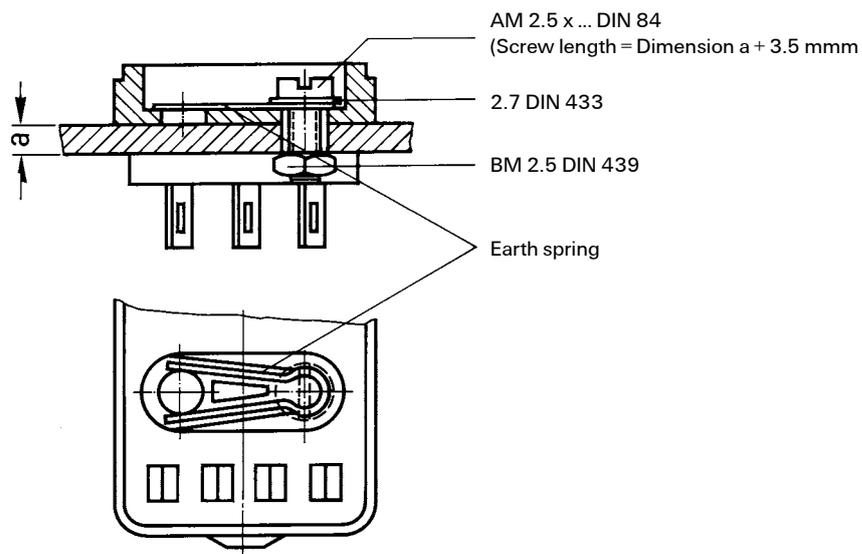
Direct mounting of relays without socket requires a fixing nut M2.5 DIN 934-m6AU.
